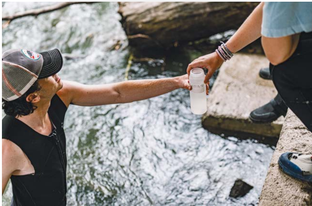
Eventually, the students will take these samples to the lab, dry them out, and weigh the solid material. This sort of data allows them to estimate how much sediment, formerly trapped behind the dam, is now mobilized by the dam removal.
